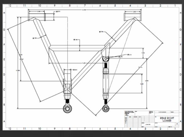
The suspension and chassis sub-team will fabricate linkages and reinforce bent members. These components will be made out of 1020 DOM steel tubing.
